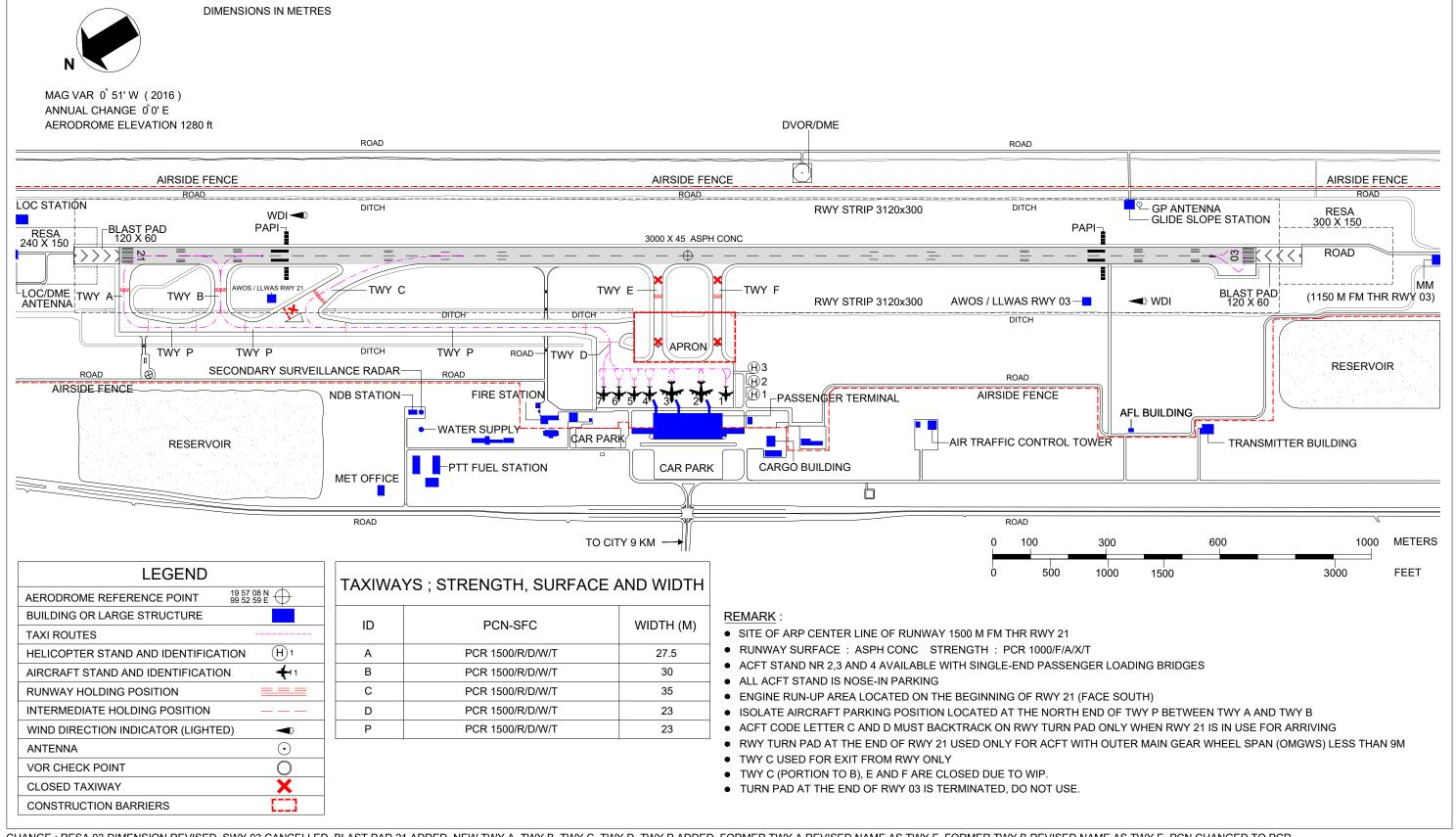
CHANGE: RESA 03 DIMENSION REVISED. SWY 03 CANCELLED. BLAST PAD 21 ADDED. NEW TWY A, TWY B, TWY D, TWY P ADDED. FORMER TWY A REVISED NAME AS TWY F. FORMER TWY B REVISED NAME AS TWY E. PCN CHANGED TO PCR
