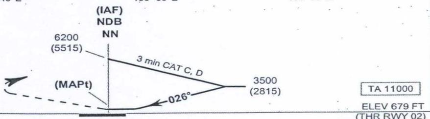
**MISSED APPROACH:** No turn before MAPt. Climb on Bearing-026 until 3500 FT then turn right direct to NN NDB at 6200 FT and hold or as directed by ATC.
