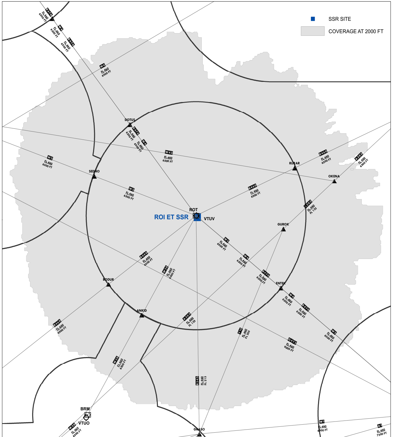
Area of Theoretical SSR Coverage Figure ENR 1.6-J - Roi Et SSR Station Coverage at 2000 FT
