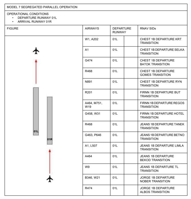
9.4 For air traffic management and effective traffic flow, runway 19L and 01L shall be mainly used for departure while runway 19R and 01R shall be used for arrival. The use of runway different from this requirement may be possible as considered necessary under special circumstances, such as adverse weather conditions or operational necessity, in normal situation, only when traffic permits ATC may initiate pilots to depart and land on the appropriate runway.
