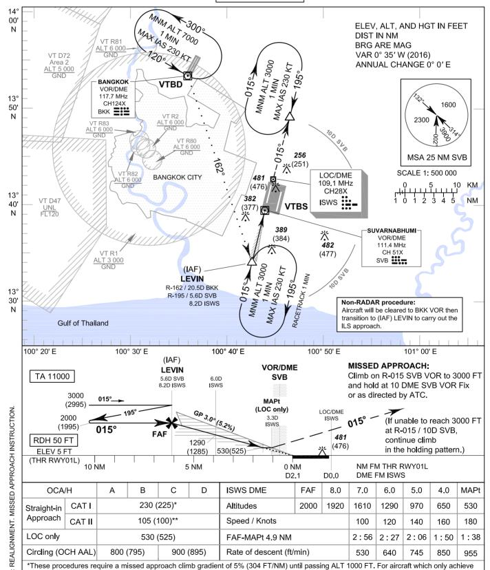
\*\*These procedures require a missed approach climb gradient of 4% (243 FT/NM) until passing ALT 1000 FT. For aircraft which only achieve
